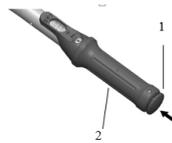
Push the locking button (1) back into the end of the handle (2). Attention should be paid to ensure that the locking button (1) engages properly. Only then is the torque safe.
