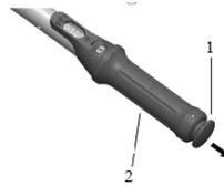
Pull out the locking button (1) on the end of the handle (2).
