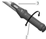
Turn the handle (2) until the desired torque in the particular scale (3) N·m or lbf·ft / lbf·in is identical with the mark in the reading glass.
